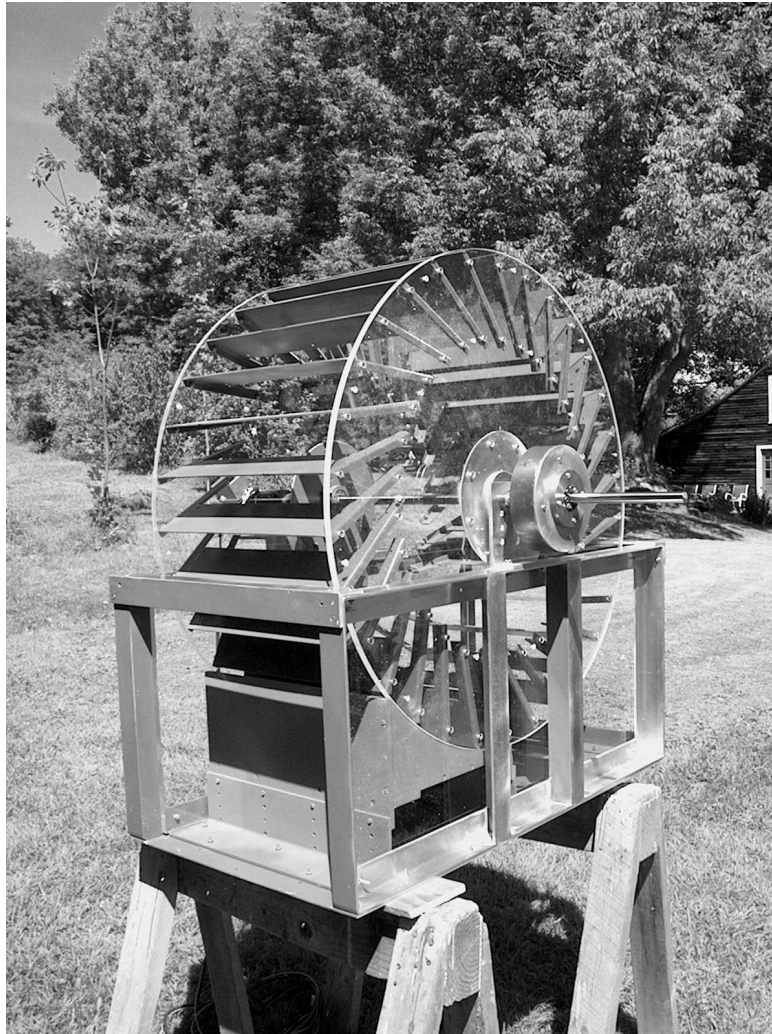
Figure 2 Prony Brake drum on side of Sagebien Waterwheel Cassette
